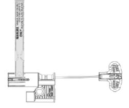
DO NOT OVER TIGHTEN. MAKE SURE GREEN IF CYLINDER IS NOT PUNCTURED, REPLACE REMOVE CYCLINDER, INSPECT CYLINDER CYLINDER FIRMLY IN INFLATOR. INDICATOR IS DISPLAYED FACE FOR PUNCTURES. STEP 3.
