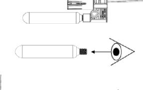
POUR DÉCELER TOUTE PERFORATION. SI LA BOUTEILLE N'EST PAS PERFORÉE, REPLACEZ-LA FERMEMENT SUR LE DISPOSITIF RETIREZ LA BOUTEILLE ET INSPECTEZ LA SURFACE NE SERREZ PAS TROP. DE GONFLAGE.
